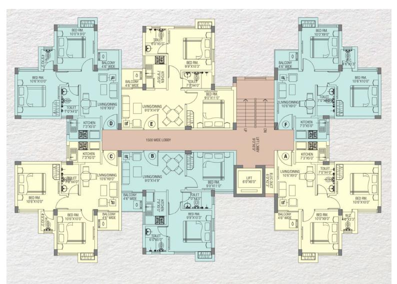
PLAN-1 TYPICAL FLOOR PLAN (1ST TO 4TH FLOOR) Madhubasant – 6 Madhuvanti – 14
